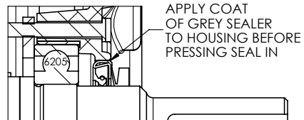
PULLEY END DETAIL
